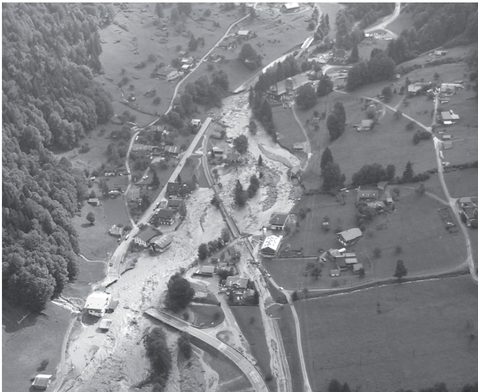
FIGURE 8. The village of Lütshental on the Schwarze Lütshine (near Grindelwald, Canton of Berne). Lateral erosion occurred because of heavy deposition, leading to bridge collapses. Destabilisation of boulder structures in the steeper reach of the background was at the origin of deposition and induced also a strong meander tendency
