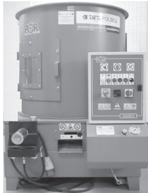
Photo 2. The hydraulic piston briquetting machine JUNIOR
