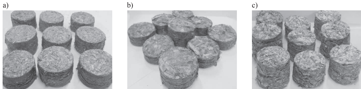
Photo 3. Briquettes produced from the tested plant raw materials: a) wheat straw, b) maize stover, c) Sida stalks
