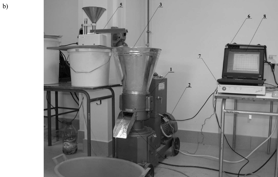
Fig. 1. The SS-4 stand: a) schema of the stand: 1 – working system of the peletizer with the flat matrix, 2 – electric engine driving the peletizer, 3 – cover up the material, 4 – pour out of the pellets, 5 – vibratory feeder, 6 – universal measure to the measurement of the power consumption, 7 – record- keeper Spider 8, 8 – the PC computer, b) the view of the stand
