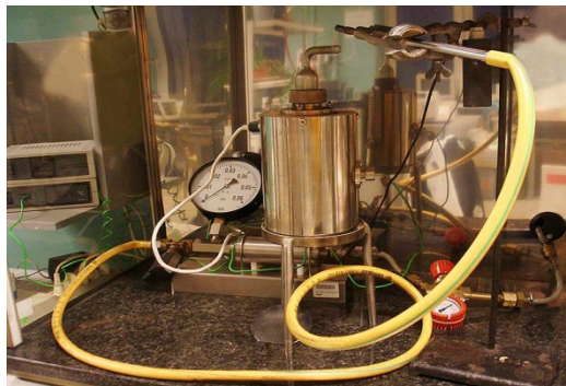
Fig. 2. Apparatus for the determination of ignition temperature of dust cloud
