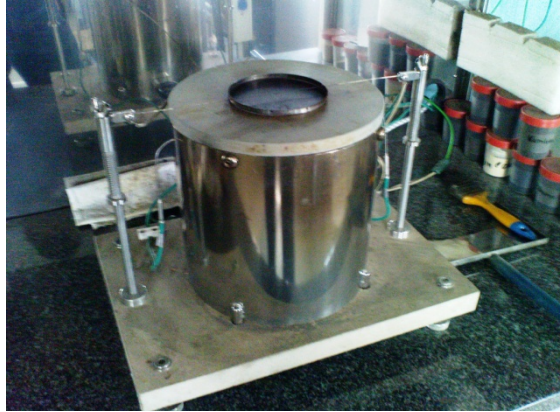
Fig. 1. Apparatus for the determination of ignition temperature of dust layer
