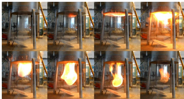
Figure. 6. Ignition of a dust cloud during experimental part
