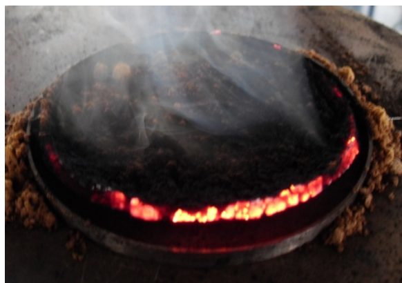
Figure. 5. Ignition of a dust layer during experimental part
