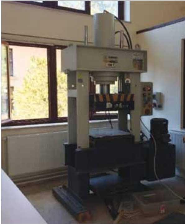
Figure 2. Hydraulic press used in densification processes
