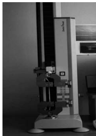
Fig. 2. Universal testing machine type Zwick BDO-FBO0.5TH.
