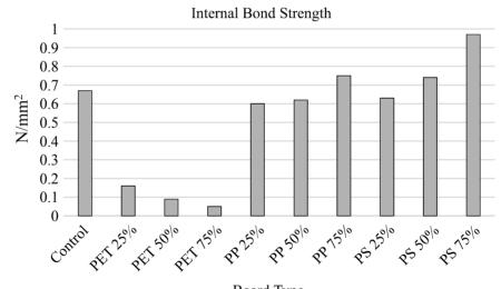
Board Type Fig. 6. Internal bond strength values of tested boards
