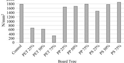
Fig. 5. Modulus of elasticity values of tested boards
