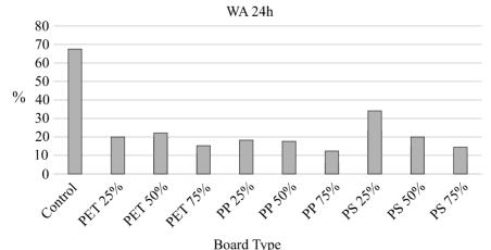
Fig. 2. 24 h water absorption values of tested boards
