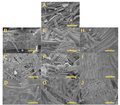
Fig. 7. SEM micrographs of boards (A: control, B: 25% PET, C: 50% PET, D: 75% PET, E: 25% PP, F: 50% PP, G: 75% PP, H: 25% PS, I: 50% PS, J: 75% PS)
