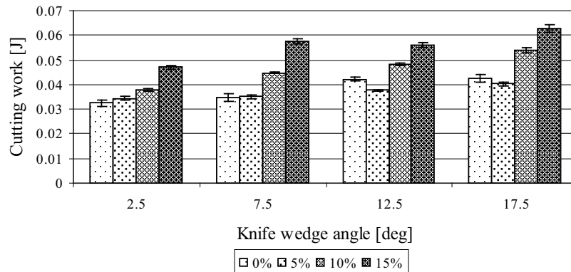
Fig. 3. Relation of cutting work of sponge-fatty cake with different addition of oatmeal to knife wedge angle
