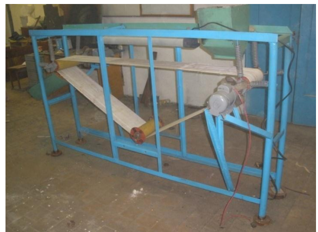
Fig. 2. The general view of the researched model of infrared vibrowave conveyer dryer.
