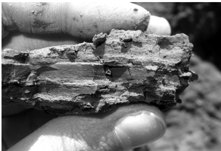
FIGURE 1. Varved clay and its laminated structure
