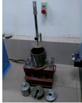
FIGURE 4. Vibrating table with weights: guide with lid 2.906, 5.017, 7.085, 10.092 kg
