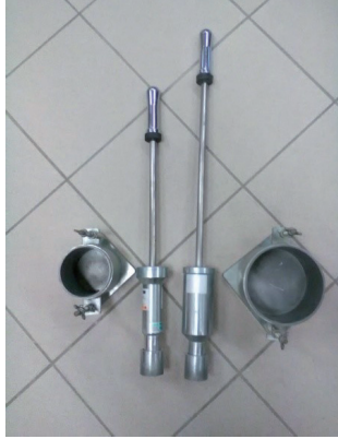
FIGURE 3. Proctor manual compactors and cylinders (on the left: A+A, on the right: B+B)
