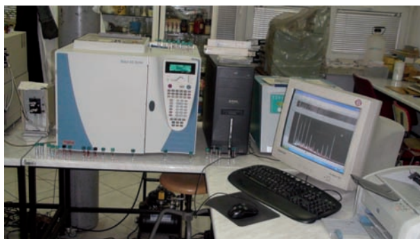
Fig. 1. The test stand equipped with a multi-channel gas chromatograph from Thermo TRACE GC Ultra type
