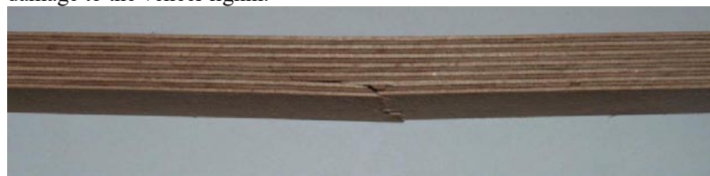
Fig.3. A sample following bending strength test
