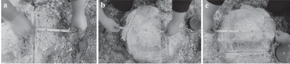
FIGURE 6. Exemplary measurement on stump after felling: a – length of under-cut (depth of under-cut), b – length of felling cut, c – width of felling cut (diameter of felling)
