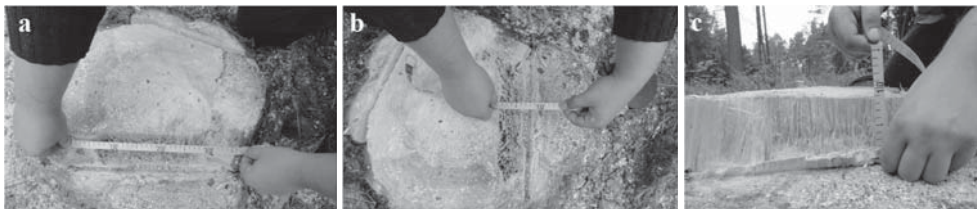
FIGURE 5. Exemplary measurement on hinge parameters: a – length, b – width, c – height
