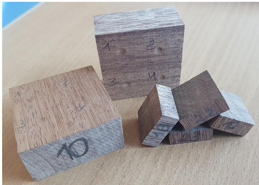
Figure 3. Samples used for the total and partial shrinkage test and for the Brinell hardness test.
