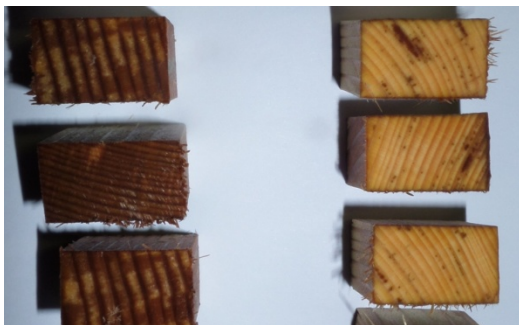
Fig. 1. The penetration of copper is detected visually with brown complex \text{Cu}_2[\text{Fe}(\text{CN})_6] . In the left column are three control Norway spruce wood specimens impregnated with a solution of copper(II) sulphate pentahydrate and on the right are three specimens which were first treated with laccase and then impregnated with a copper solution
