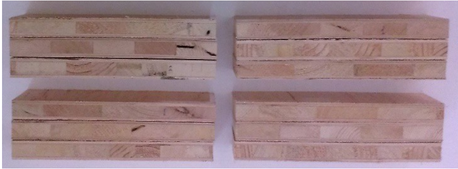
Fig. 7. Specimens of veneered BB with the core-board from PCW to test the static-bending strength across strips
