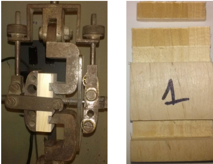
Fig. 16. Test specimen of the PCW-BB for shear strength at the moment of load
