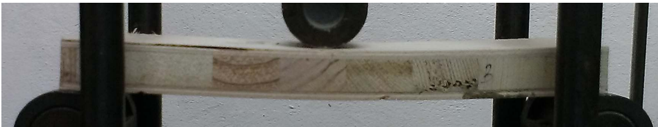
Fig. 10. Test specimen of the PCW-BB for bending strength at the moment of load
