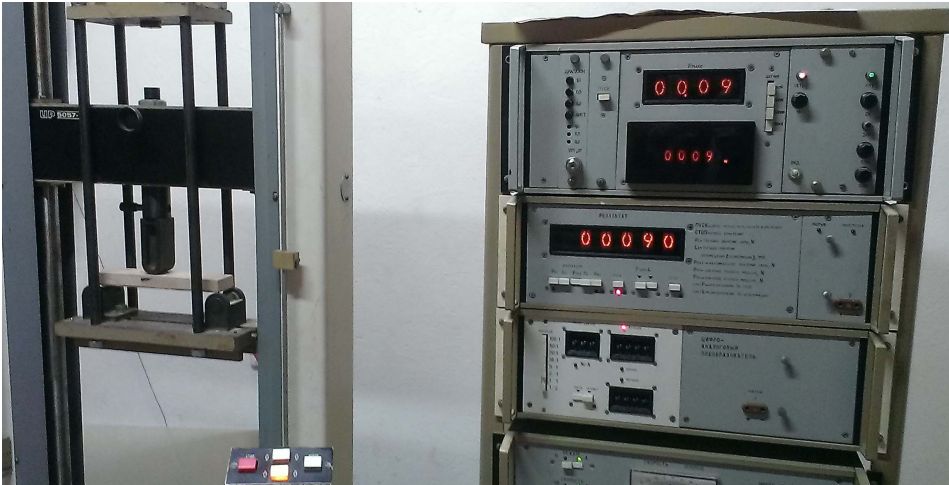
Fig. 9. The laboratory test machine IP5057-50 (maximum load – 50 kN)
