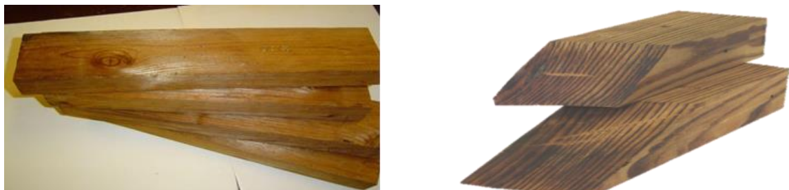
Figure 5 - Samples after drying and thermal modification.
