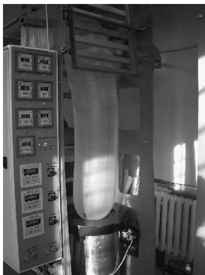
Fig. 1. TPS film blowing in KIP laboratory [8]
