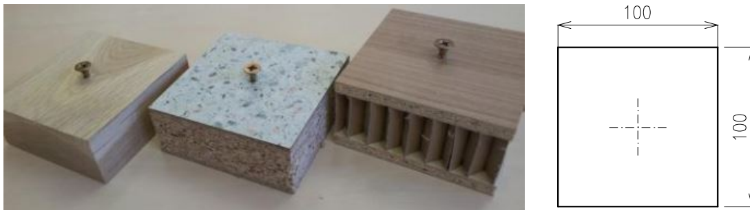
Fig. 1. Test specimens - material, shape and dimensions
