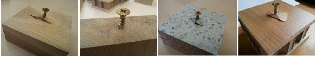
Fig. 4. Demonstration of damage of the test specimens for screws 6 x 40 mm loaded by axial force
