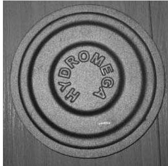
Fig. 6. Semi-finished castings of the planetary gear
