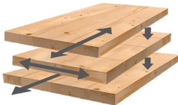
Figure 2. CLT structure ( Global Warming, Carbon Dioxide, Buildings and CLT! - New Materials & Applications / New Materials & Applications (elsevier.com) ).
