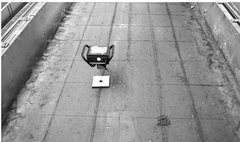
FIGURE 1. The Penetrologger cone penetrometer in the soil channel with marked places of compaction measurement places
