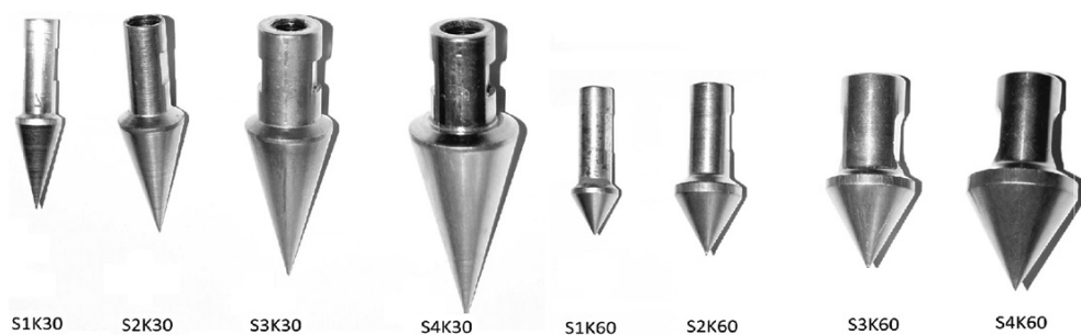
FIGURE 2. Cone shaped end pieces of Penetrologger penetrometer (S – identification connected with the cone base area, K – cone apex angle)
