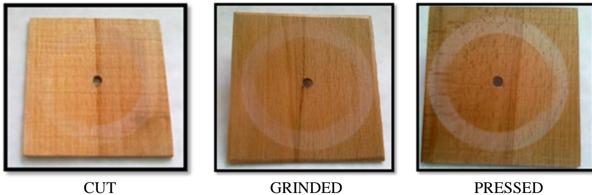
Figure 2. The traces after abrasion resistance test visible on the thickest coating film of WAX surface finish on cut, grinded, and pressed wood surfaces.
