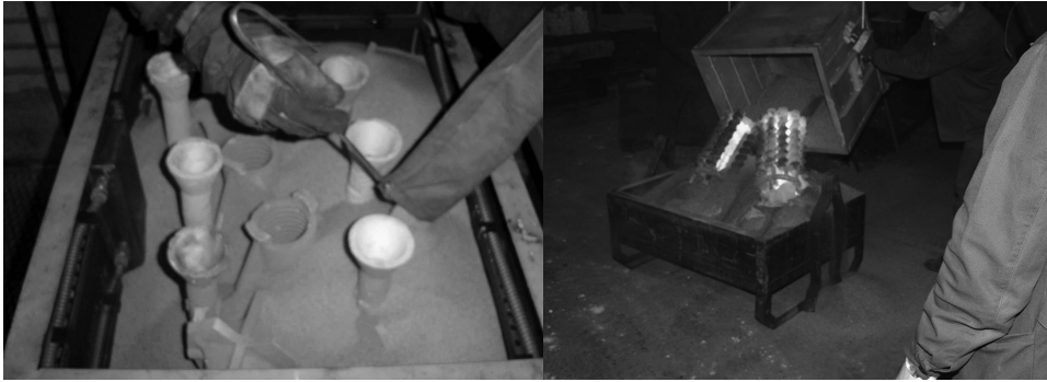
Fig. 8. Pilot castings, a - set of polystyrene patterns, b -in raw condition after pouring
