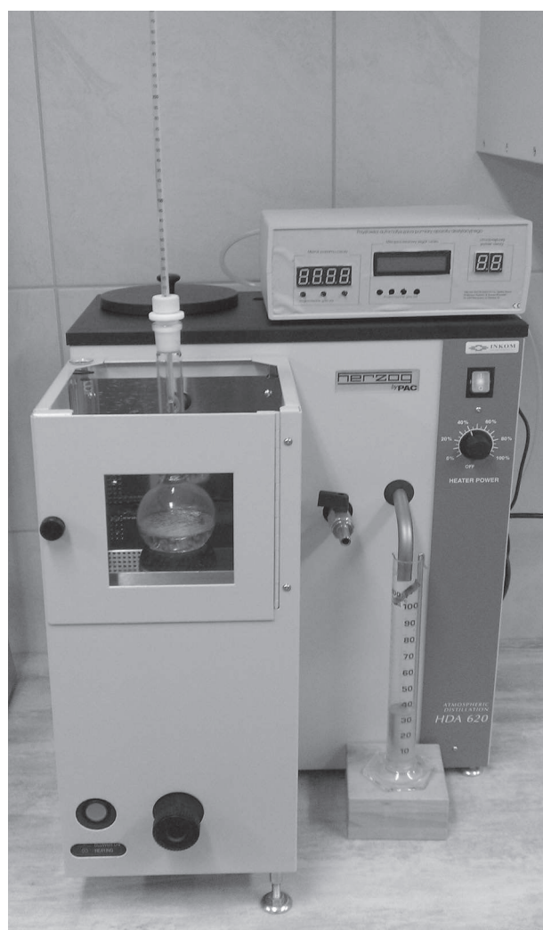
Fig. 2. Photo bench equipped with a distiller HAD 620/1 by Herzog
