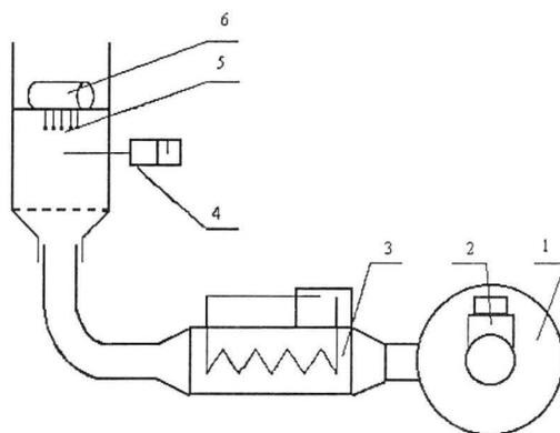
**Fig 1.** Scheme of measuring stand: 1 - fan, 2 - control damper, 3 - heater with a temperature controller, 4 - thermoelement, 5 - filaments with droplets, 6 - cylinder.
