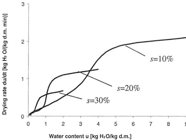
Fig. 3. Drying rate versus water content for different extract content in concentrates of barley malt extracts.
