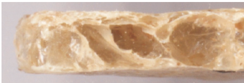
Fig. 5. Structure of gluten membranes thermally set – cross section of gluten sample.
