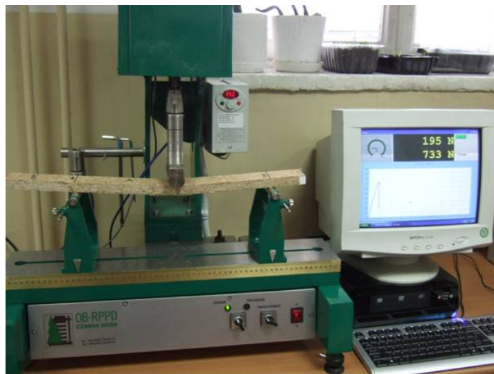
Fig. 1 Stand for testing MFP specimens in bending
