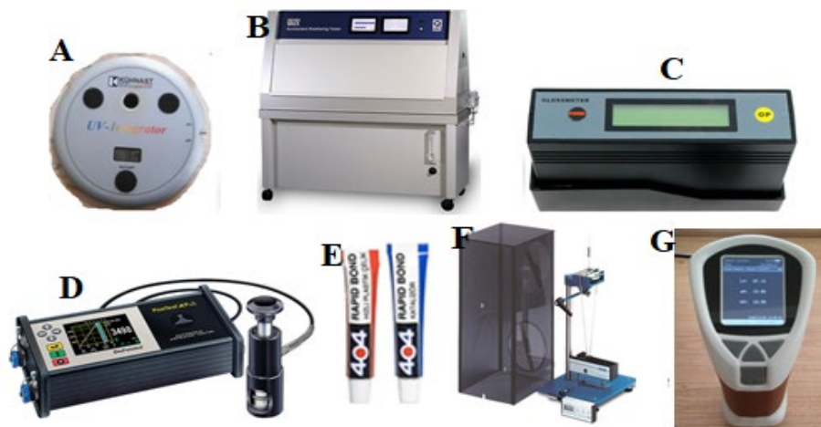
Fig. 1. UV integrator (A), accelerated weathering machine (B), gloss meter (C), pull-off adhesion tester (D), adhesive glue for surface adhesion test (E), pendulum hardness testing device (F), and colorimeter (G)
