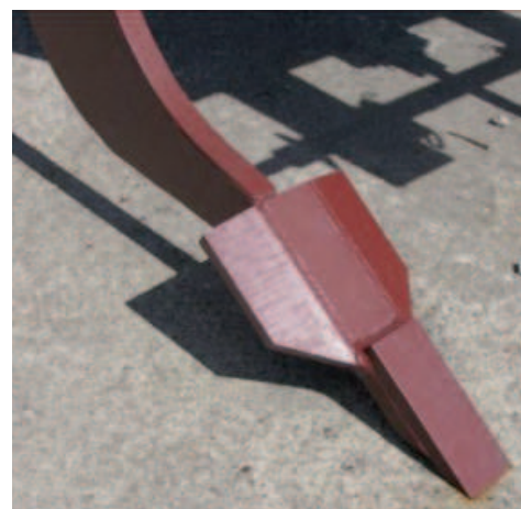
Fig. 5. A photograph of the welded subsoiler coulters
