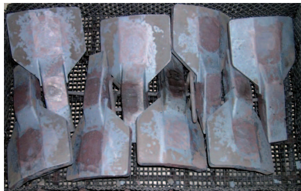
Fig. 9. Subsoiler coulters cast by the developed technology
