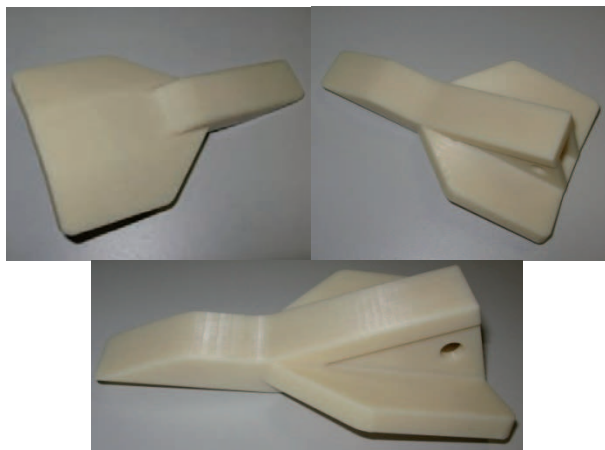
Fig. 7. Pattern of subsoiler coulter made by RP on a 3D DIMENSION 1200es printer
