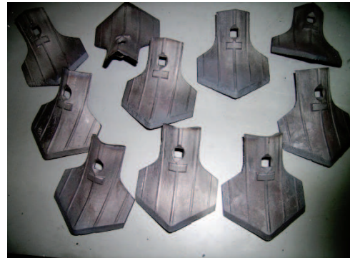
Fig. 4. Duckfoot castings for the cultivator spring teeth (made by the developed technology)
