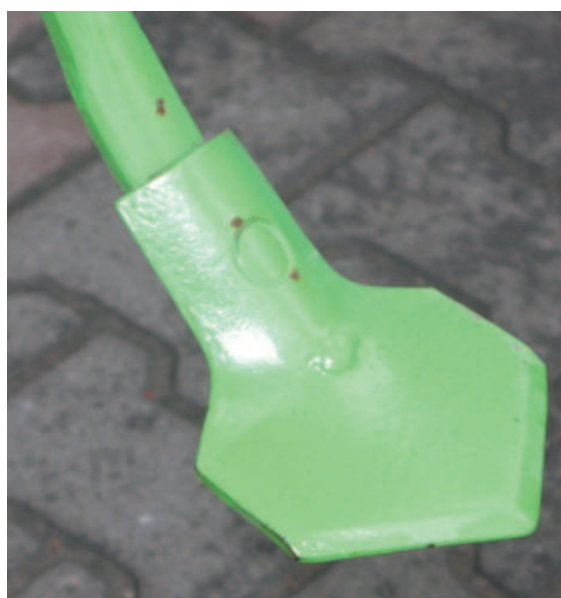
Fig. 1. A photograph of forged duckfoot for the cultivator spring teeth
