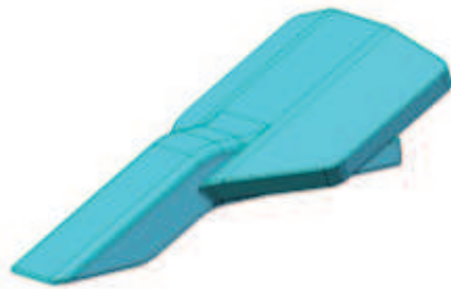
Fig. 6. Virtual 3D model of subsoiler coulter made in Solid Works
