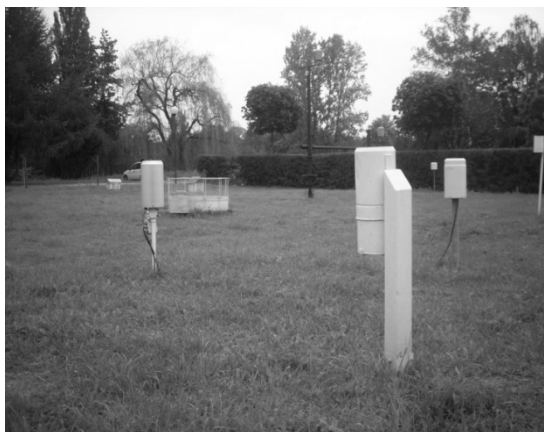
FIGURE 2. Telepluviometer and Hellmann rain gauge at the Warsaw Ursynów station
