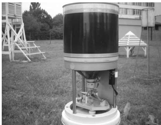
FIGURE 1. Measurement unit in the telepluviometer
