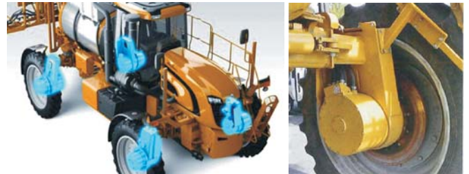
Rys. 7. Samobieżny opryskiwacz AGCO ElectRoGator 1386 [2, 5] Fig. 7. AGCO ElectRoGator 1386 electrically powered high-clearance sprayer [2, 5]
