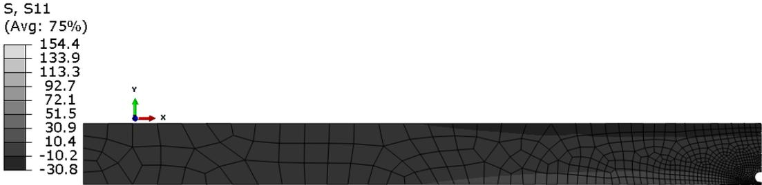
Figure 4. Normal stress distribution ( $\sigma_{11}$ ) and the mesh of  $\frac{1}{2}$  of the reinforced beam
