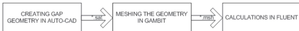
Fig. 2. Stages of building the model of the variable-height gap in the CFD Fluent package
