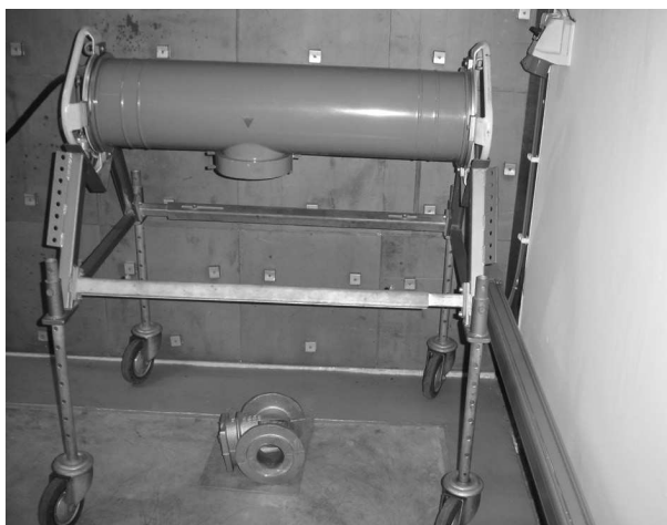
Fig. 4. Corps cast DN 150 in the X-ray stand
