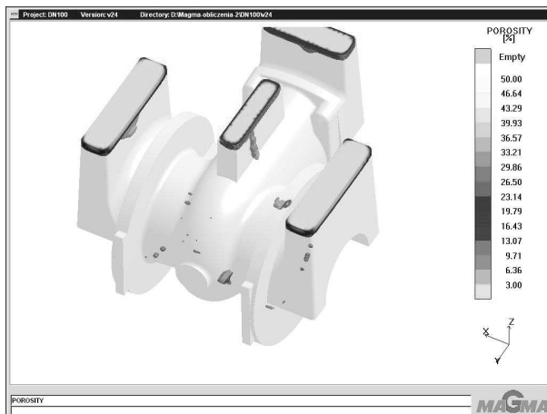
Fig. 3. The predicted sites of porosity in the valve corps cast DN 80
