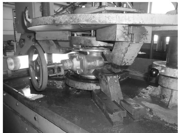
Fig. 5. Test of seal-tightness of the valve (in water)
