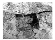
Fig. 1. Detail of photo-degraded surface and rotten area
