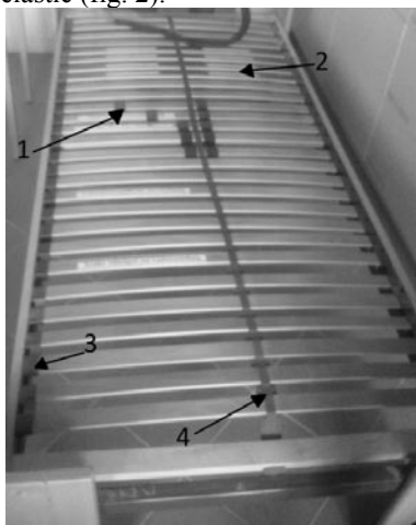
Fig. 1. The frame used in the research; 1 - elements tying the elastic battens, 2 - battens with increased elasticity, 3 - rubber handles, 4 - middle strap (own elaboration)
