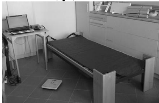
Fig. 3. The test stand for the study of the quality and the distribution of contact stress (own elaboration)
