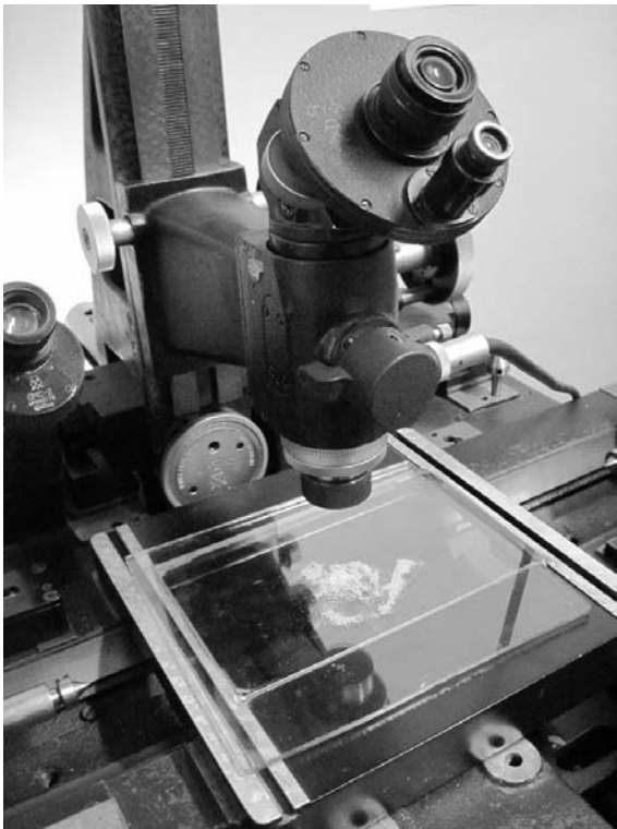
Fig. 4. The universal measuring microscope UIM-21
