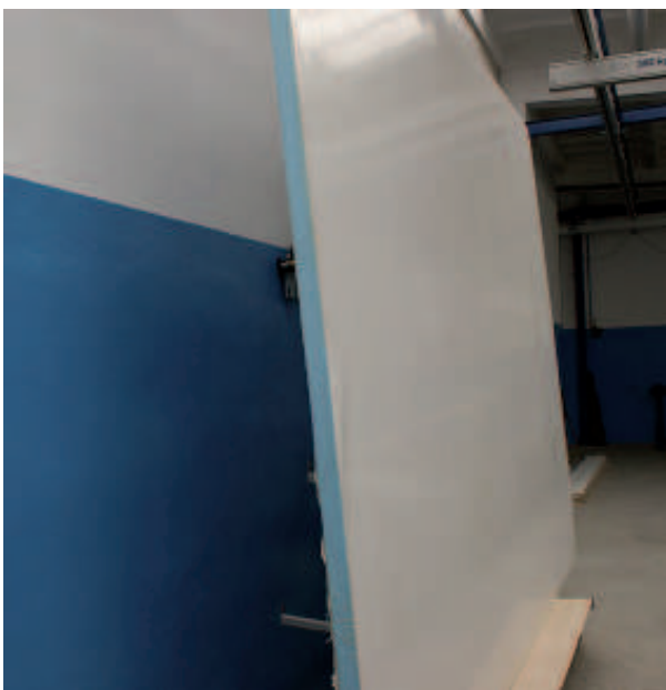
Fig. 11. The composite panel produced with implementation of the vacuum adhesion technology
