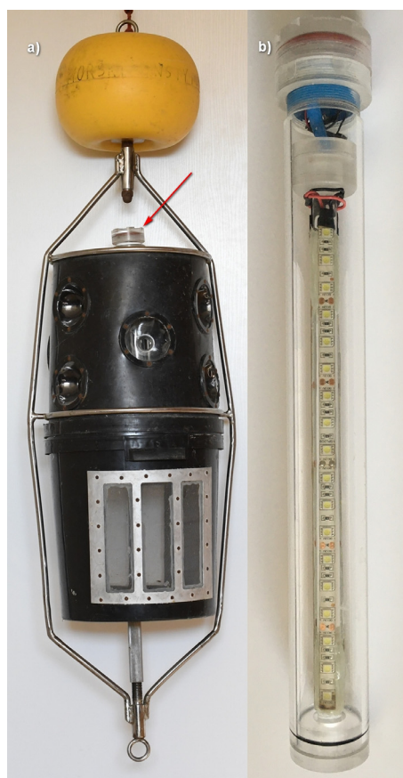
Figure 2 Light trap used in this project: a) overall look; b) light module. The arrow indicates the location of the battery compartment cap of the light module.
