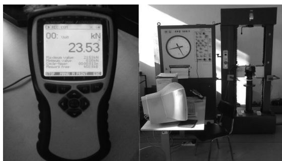
Fig. 3 The ALMEMO measuring device and the FPZ 100/1 tensile testing machine
