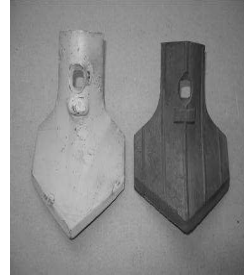
Cast subsoiler coulters. Cast duckfoot for the flexible cultivator teeth
