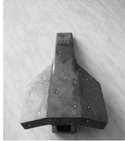
Cast subsoiler coulters. Cast duckfoot for the flexible cultivator teeth
