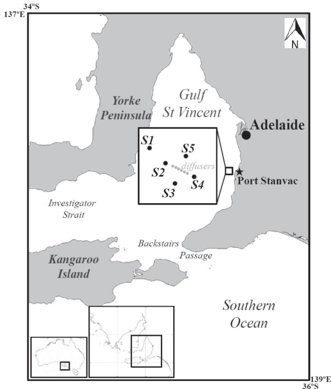
Figure 1. Map of the sampling area in the Gulf St Vincent (South Australia). Samples were taken at the intake pipe (S1) and at 100–150 m from the outfall diffusers (S2–S5) of the desalination plant. The intake pipe and the outfall saline concentrate diffusers are located 1500 m and 1100 m respectively away from the coastline where the desalination plant was built
