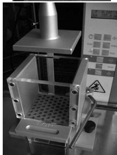
Fig. 1. Test adapters for texture measurements: a) Warner-Bratzler's knife, b) OTMS – Ottawa cell
