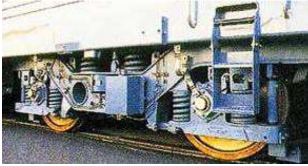
Fig. 8. Running part of the Prima locomotives
