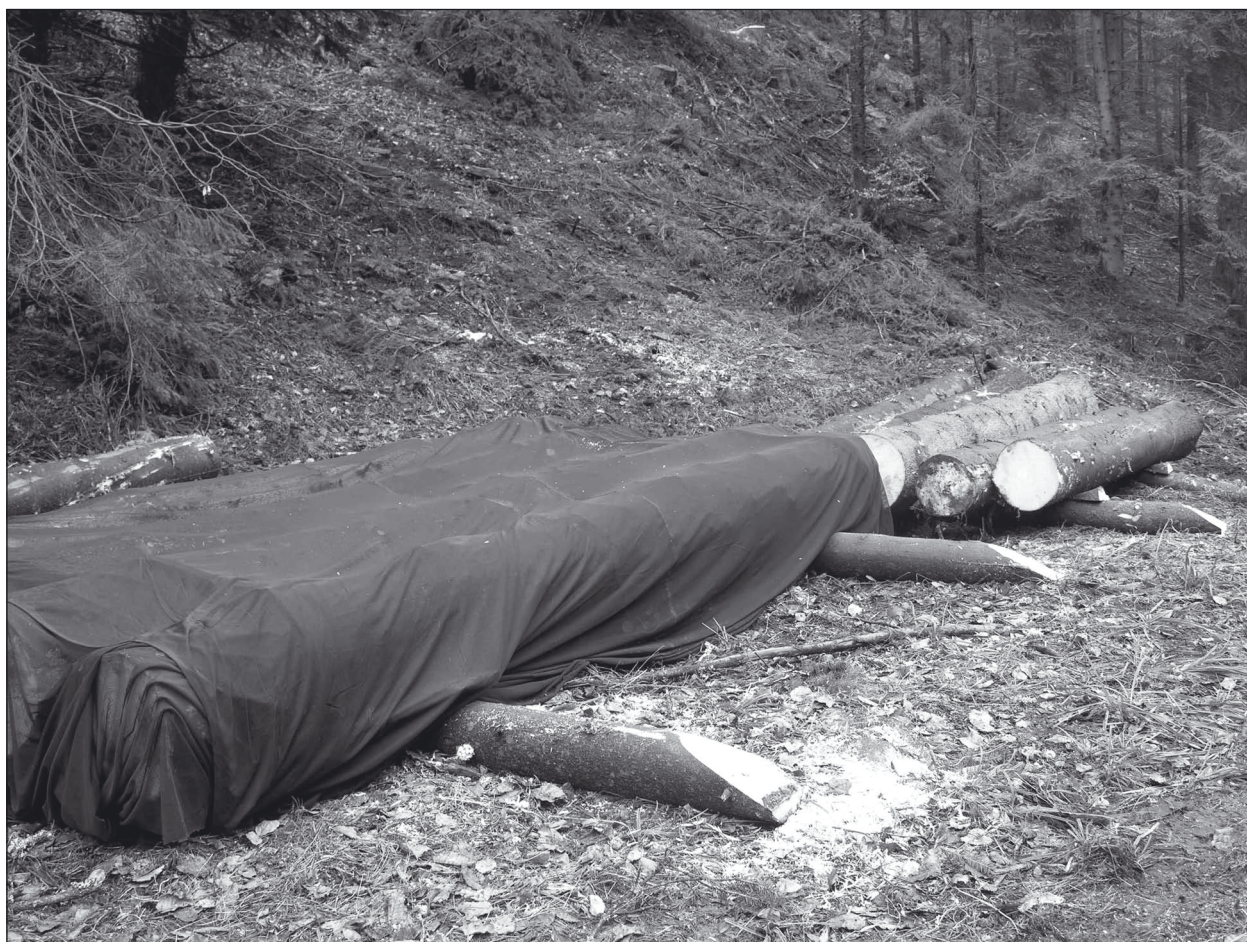
Fig. 1. The logs wrapped in Storanet® and control (not wrapped) logs
