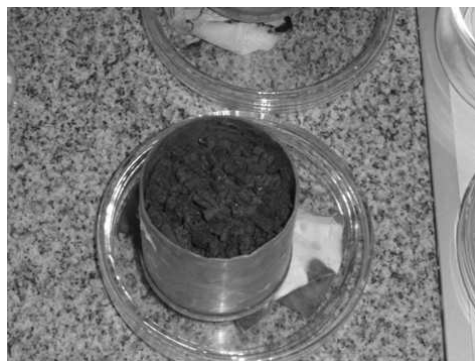
FIGURE 3. The sludge in soil sampling cylinders
