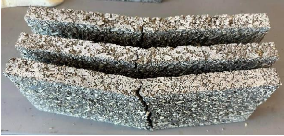
Fig. 3. Samples for MOR and MOE testing - after the test.
