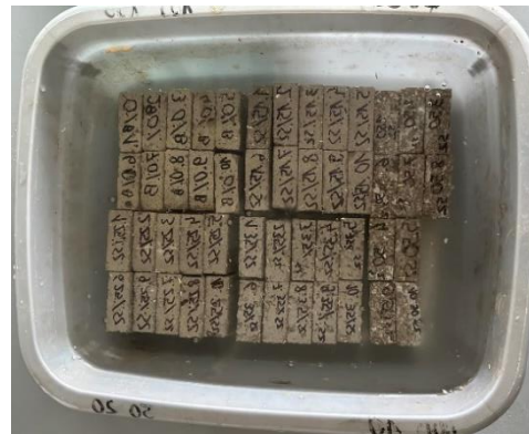
Fig. 5. Thickness swelling and water absorption test samples.
