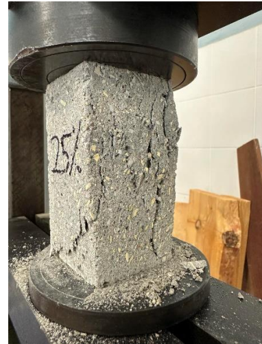
Fig. 4. Compressive strength test sample during testing.
