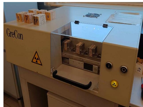
Figure 2. Density profiler X-ray by GreCon
