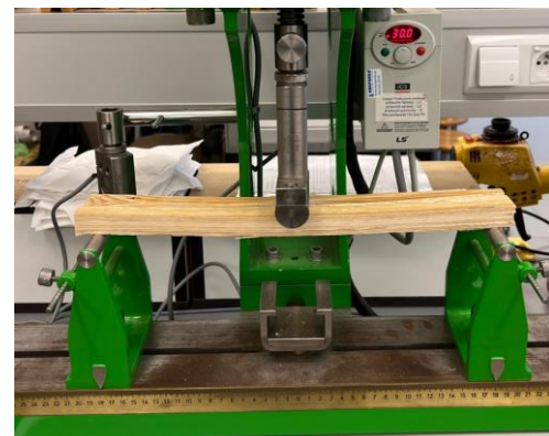
Figure 3. Sample during MOR and MOE testing
